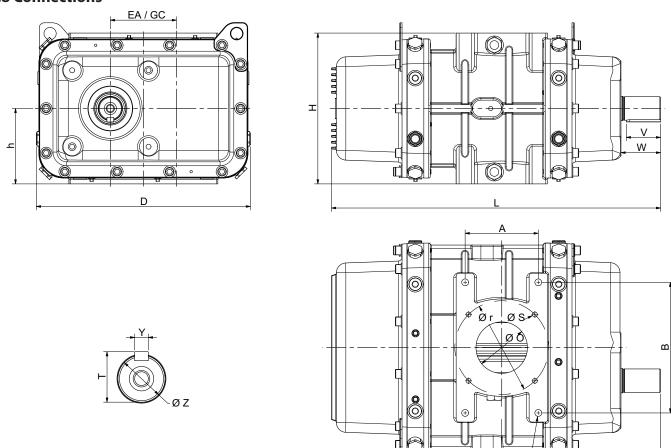
Figure 3 - Left and Right Hand blower dimensions
