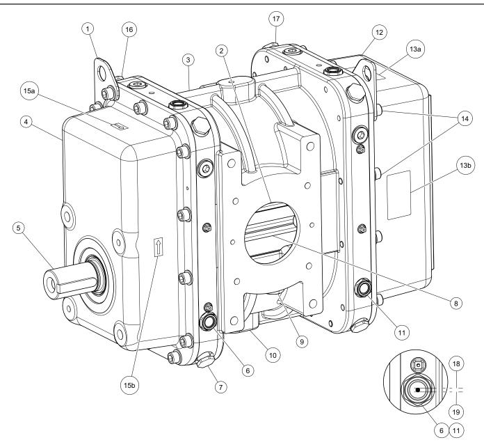
Figure 1 – Components of the PTB blower
